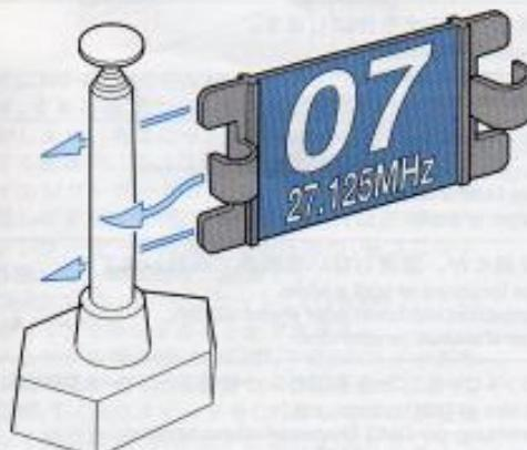
The frequency flag is used as an easy means of frequency identification. It should be attached to the antenna as shown. Please note that using the same frequency at the same time can cause serious accidents.
