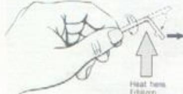
Cut runner into a short length. Heat as shown. Remove from flame and stretch both ways. Allow about 15 seconds to cool. Make two 14cm long. Take care when using fire.
